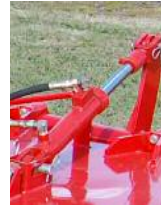
Hydraulic two position diverter valve, for the wing folding or the raising of the machine during work.
